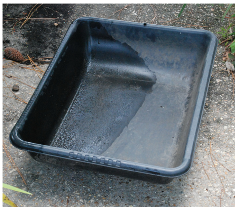
A mortar mixing tub from Home Depot, six inches deep with no drain holes.
